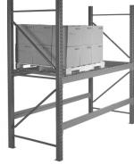
Keep space between the racks and the walls, ensure that the racks are stable and, where possible, fixed together and to the wall and/or to the floor.
