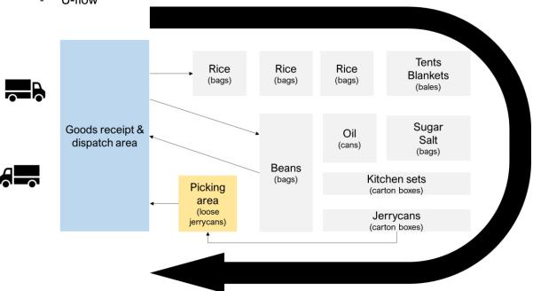
U-flow is used when the receiving and loading areas are next to each other on the same side of the building. It provides the following features:
