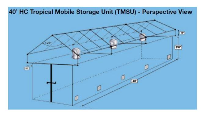
The major risks to a container storage unit are adverse weather and pests. Accurate roofing, anti-corrosion and anti-rust measures will protect against adverse weather. Netting and regular maintenance will prevent damage from pests.
